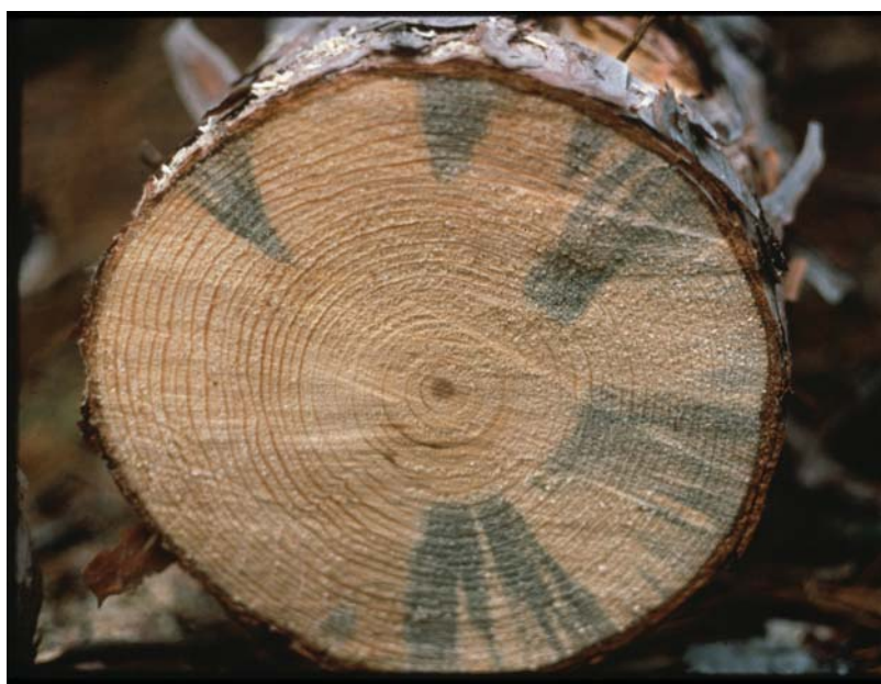
FIGURE 18.11 Cross-section of a red pine infected with blue-stain fungi. (Photo by Kier Klepzig, USDA Forest Service)
