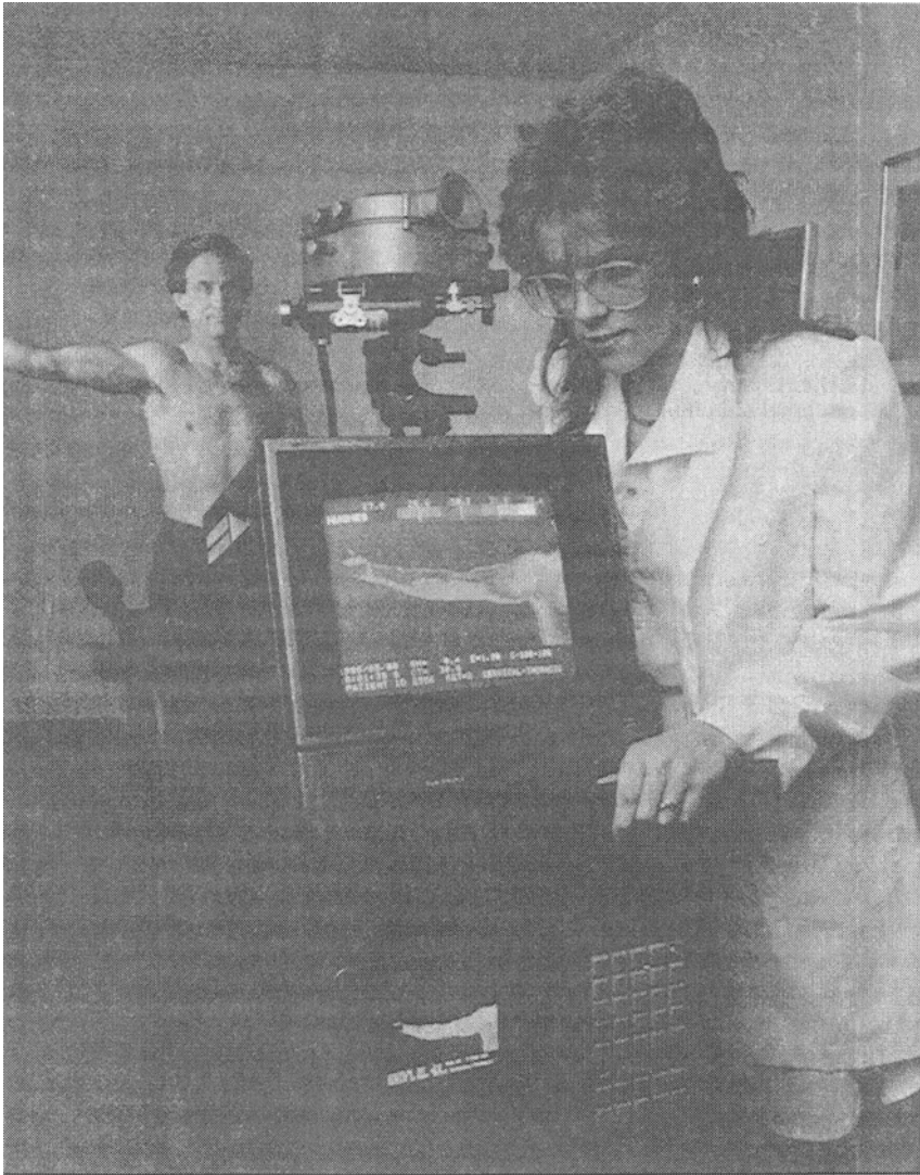
Figure 5-6. Vasodilation and constriction recorded with infrared thermography. Reproduced by permission of Hughes Aircraft Company, Carlsbad, California.
