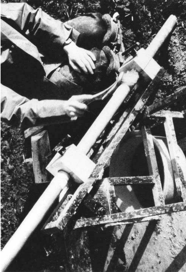
FIGURE 2.3. An auger jig system used to install angled minirhizotron tubes (from Mackie-Dawson and Atkinson, 1991).
