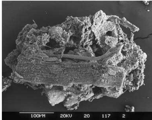
FIGURE 3.4. Scanning electron microscopy (SEM) picture of a macroaggregate (250- to 500- \mu\text{m} diameter) with particulate organic matter and hyphae (V. V. S. R. Gupta, with permission).
