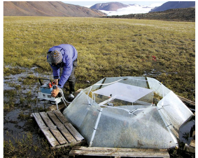
Figure 30.19 The International Tundra Experiment (ITEX) uses small, passive, clear plastic, open-top chambers to warm the tundra and extend the growing season. The chambers raise the daily temperature of the tundra plant canopy by 1.5^\circ\text{C} to 1.7^\circ\text{C} , which is in the range predicted by global climate simulations. This experiment, which has been in place in the Barrow Environmental Observatory for three years and for one year at Atkasuk, Alaska, has already provided new insights on flower and growth responses to warming.
