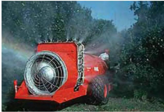
FIGURE 9-26 Application of fungicides (and insecticides) in a fruit tree orchard using a tractor-mounted, high-pressure, high-volume air blast sprayer. (Photograph courtesy of R. J. McGovern, University of Florida.)
