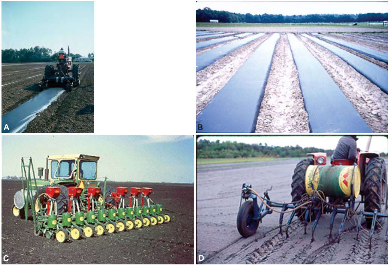
FIGURE 9-31 Equipment for application of soil pesticides and fumigants. (A) Tractor applying a fumigant and laying plastic over it to keep the chemical from early escape. (B) Field beds treated with a volatile chemical and covered with plastic. (C) Multidisk tractor used to incorporate nonvolatile granular chemicals in soil. (D) Broadcast chisel application of low-volatility liquid fumigants into soil. [Photographs courtesy of (A) R. T. McMillan and (B–D) D. W. Dickson, University of Florida.]
