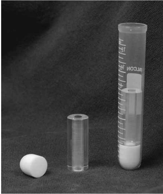
Fig. 1. Sucrose cushion apparatus. Set the poly-L-lysine-coated cover slip on top of the white bottom piece ( left ) with the coated side upward and overlay the top piece ( middle ) on them. Insert the two pieces into a Falcon 2059 tube carefully not to break the cover slip ( right ).
