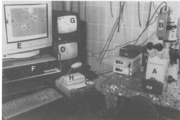
Fig. 4.4. Workstation: inverted microscope (A), video camera (B), camera control panel (C), black and white monitors (D, G), Macintosh (E), video recorder (F) and optical drive (H)
