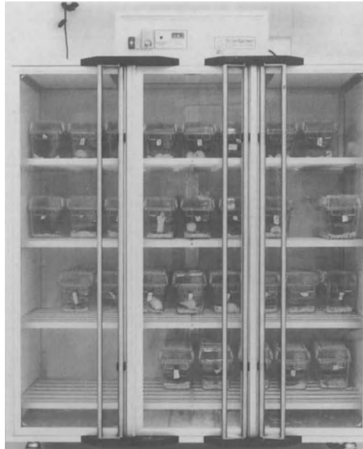
Fig. 11.2. An example of a ventilated cabinet, the Scantainer. Note the filter-top cages inside the cabinet and the air-handling unit on the top which draws the air through the cabinet
