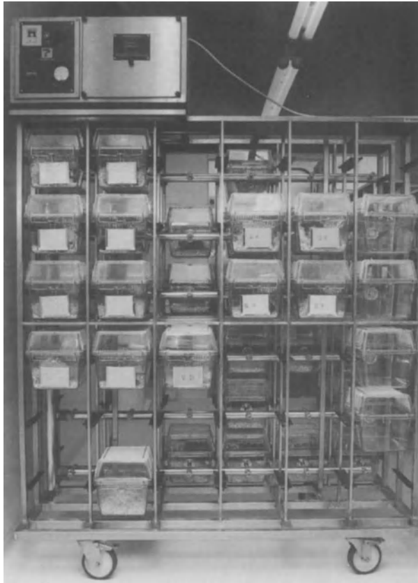
Fig. 11.4. An individually ventilated cage rack (Scanbur). The air-handling unit on top of the rack forces air into, and removes it from, each cage individually. The cages are maintained under positive pressure. Animals of different health status can be kept in adjacent cages without cross-contamination occurring
