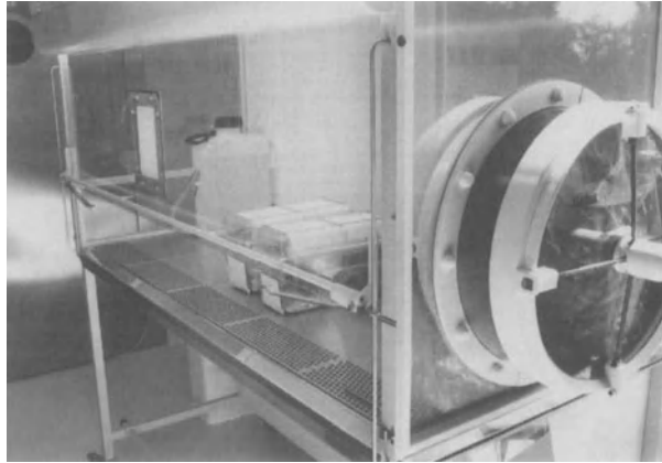
Fig. 11.3. Laminar flow hood (Holten) for use with the Scantainer. The front shield can be raised to the level indicated on the frame without compromising the sterility of the interior. Therefore the cages can be serviced and the mice examined without affecting their health status
