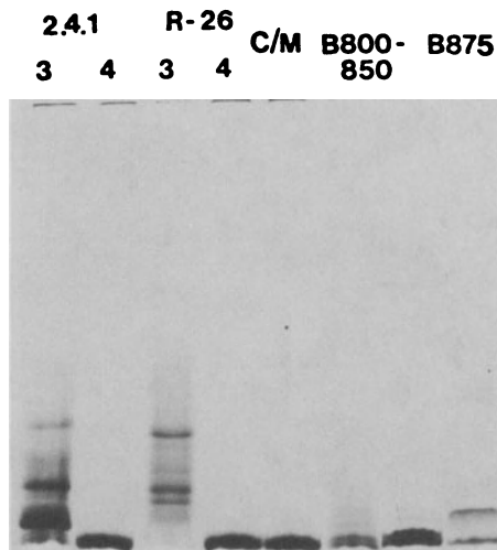
Figure 2. SDS-PAGE of light-harvesting polypeptides. Under 2.4.1: 3-B875 fraction solubilized without detergents, 4-B800-850 fraction solubilized without detergents; Under R-26: 3-875 fraction solubilized without detergents and missing B875 polypeptide, 4-B800-850 fraction solubilized without detergents; C/M, chloroform/methanol soluble B800-850 polypeptides; Under B800-850: two different preparations of spectrally active detergent solubilized complex; B875, preparation of spectrally active detergent solubilized complex.
