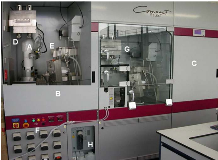
Fig. 1. The Compact Select automated cell culture platform. The inset shows an enlarged image of the manipulation chamber and pipette head. Major processing components are labeled: (a) Robot arm; (b) flask incubator; (c) plate incubator; (d) flask de-cappers; (e) flask holders; (f) media pumps; (g) pipette head; (h) Cedex-automated cell counter.
