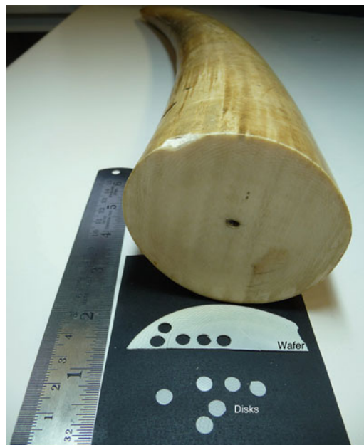
Fig. 1. Dentine wafers are cut from blocks of dentine using a low-speed diamond saw. Uniform 5-mm Ø discs are then punched from the wafer.
