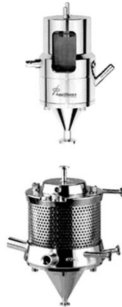
Figure 8 Ultrasonic cell separation device. The standing wave field in the resonator chamber aggregates and retains cells from the effluent stream. Periodic shut-down of the power to the resonator and effluent pump allows the aggregated cells to settle out of the resonator and into the bioreactor. (Courtesy of Attlikon.)
