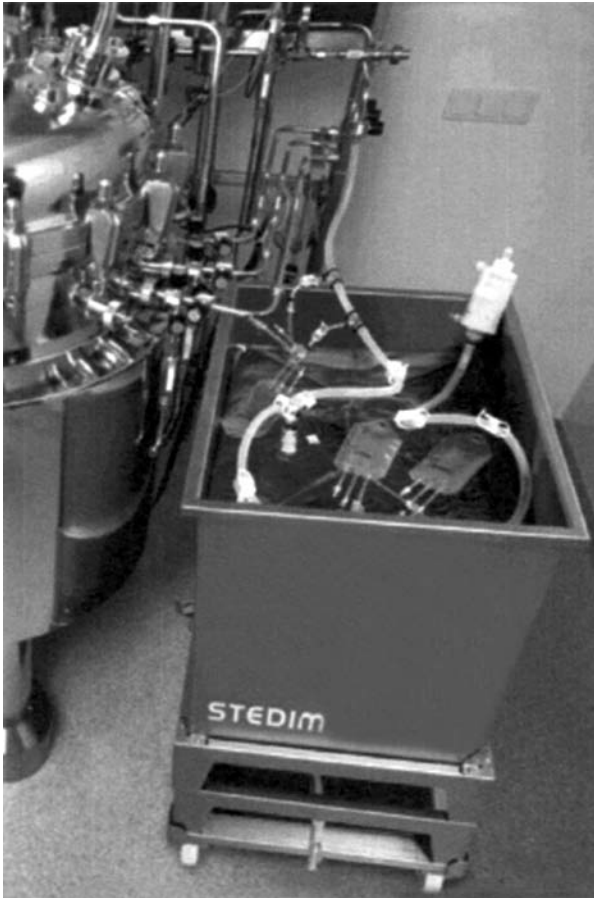
Figure 7 Stainless steel pallet tank used for holding media and buffer bags (photos courtesy of Stedim). (See color insert p. 9.)
