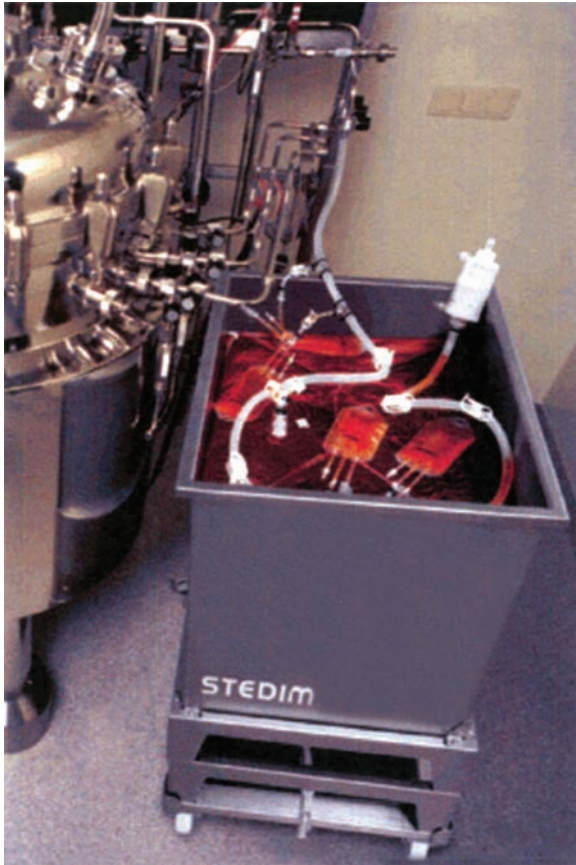
Figure 16.7 Stainless steel pallet tank used for holding media and buffer bags (photos courtesy of Stedim).
