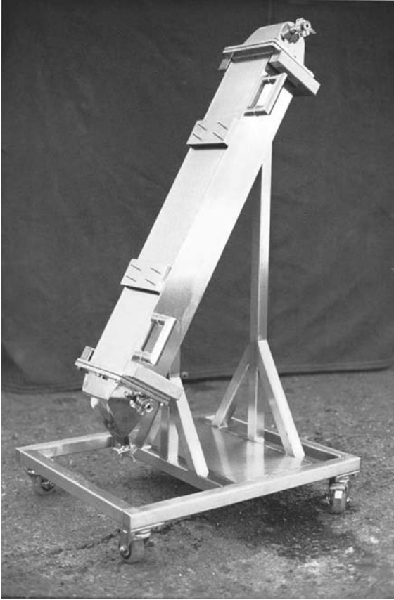
Figure 6 Inclined plate settler used at industrial scale cultivation of mammalian cells. (Courtesy of Biotechnology Solutions, California, U.S.A.)
