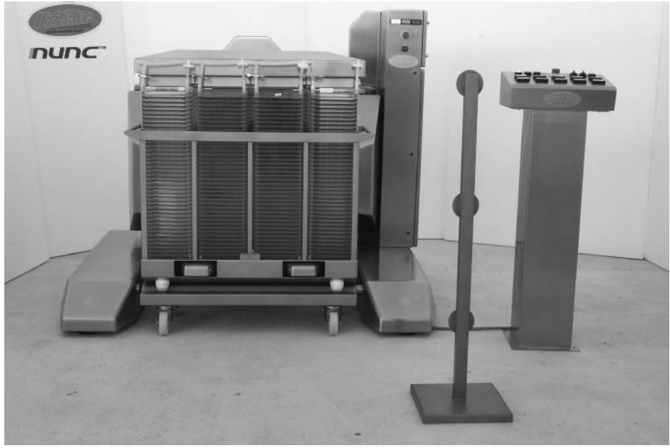
Figure 10.3 Four 40-layer cell factories on an electric handling rig (Photograph courtesy of Nunc).
