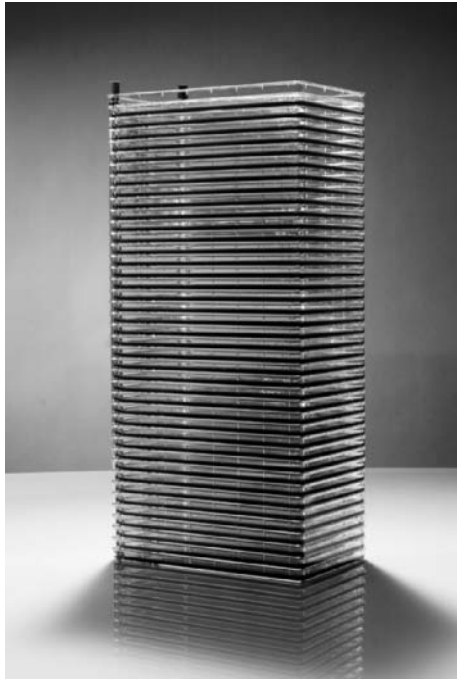
Figure 10.2 A 40-layer cell factory (Photograph courtesy of Nunc).
