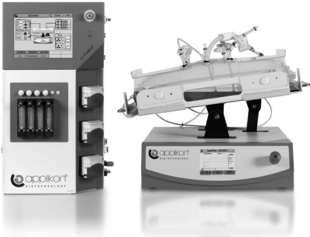
Figure 10.7 Wave-type bag system (Photograph courtesy of Applikon.).
