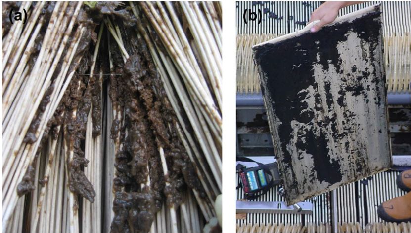
FIG. 3.9 Clogging (sludging) of MBR membrane channels in (a) a hollow fibre and (b) a flat sheet module.
