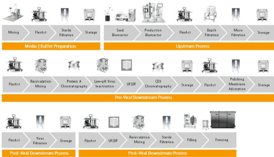
Fig. 9 Example of a generic single-use SU platform for bulk production of mAb
