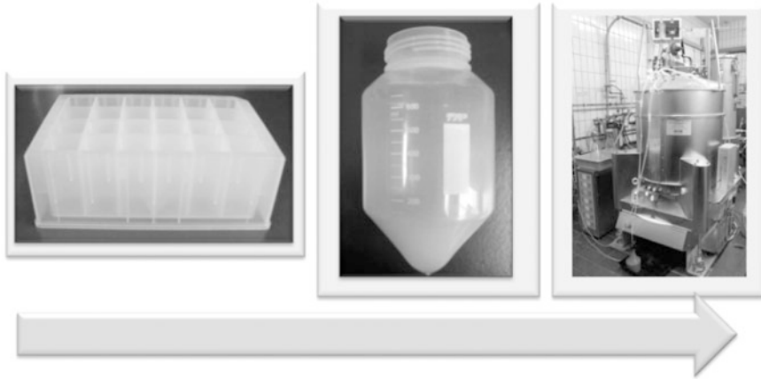
Fig. 10 Scale-up from deep-well plates to TubeSpin 600 bioreactors and finally to Kuhner SB200-X orbital shaking reactors
