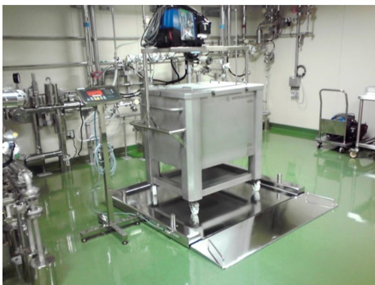
Fig. 4 Common solution: Palletank ® on Sartorius IFS4 flat-bed scale with a ramp
