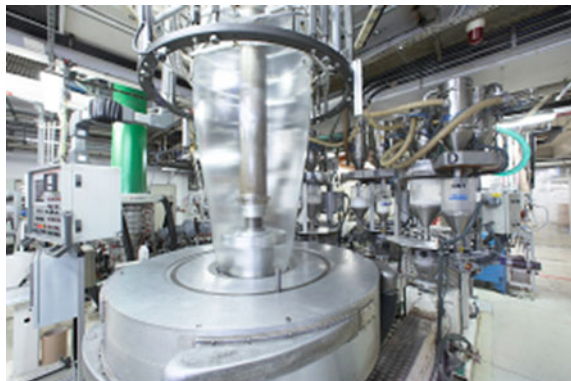
Fig. 2 Blown film extrusion (Courtesy of Südpack GmbH)
