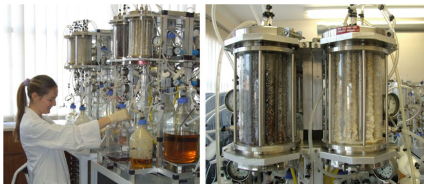
Fig. 1 Modular scale-up. Streptomyces sp. (left) and Penicillium sp. (right) cultivated in reusable Quorus Bioreactor for the production of bioactive small molecules under Synexa Life Sciences in the mid-2000s
