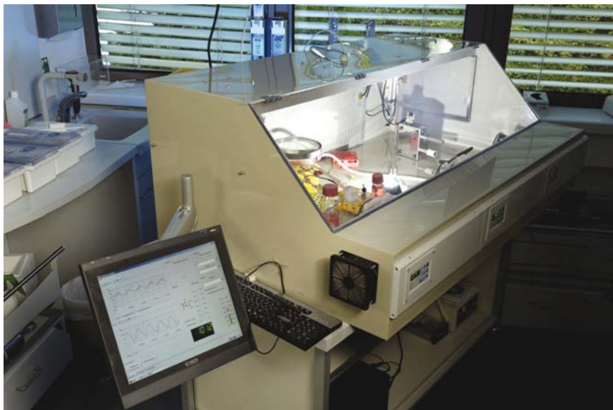
Fig. 4 A computer-based bioreactor system for vascular tissue engineering developed at the Fraunhofer IGB. The figure shows the whole bioreactor system. The bioreactor described in Fig. 3 is inserted into a climate chamber. A computer simulation forms the basis of the fluid dynamics of the bioreactor system to control the hydrodynamic regime and temperature. The medium flow through the growing vascularised tissue is provided by a roller pump in the same way as the heart pumps blood through the human circulatory system. The computer regulates the arterial oxygen and nutrient supply via parameters such as blood pressure, temperature and flow rate
