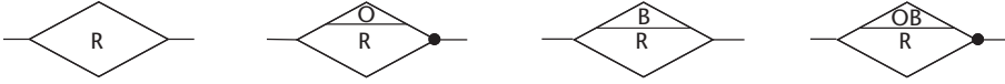
Figure 3.4 EER notations for unordered set, ordered set, unordered bag, and ordered bag relationships (from left to right).
