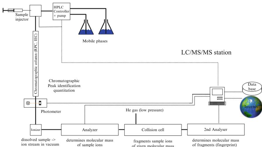
**Fig. 3.13** Liquid chromatography coupled to tandem mass spectrometry (LC/MS/MS) can be used to identify and quantify unusual compounds in biological fluids. The sample is first separated on a chromatographic column (gas chromatography may be used for volatile compounds), and then the mass of compounds is determined by MS. Finally, the fingerprint spectrum of each compound of interest is determined. Together, these data identify a compound “beyond reasonable doubt” even in court
