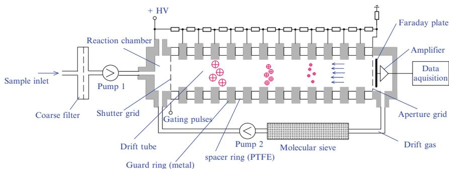
**Fig. 3.12** The ion mobility spectrometer is used to detect and identify contaminants in air, for example, agents of biological or chemical warfare. Sample molecules are ionised and move against a stream of drift gas. Small molecules will experience less resistance and arrive at the FARADAY plate earlier than large molecules. The entire system (computer, gas supply etc.) can be mounted onto a small vehicle and used for real-time analysis, say, after a terrorist attack or industrial accident
