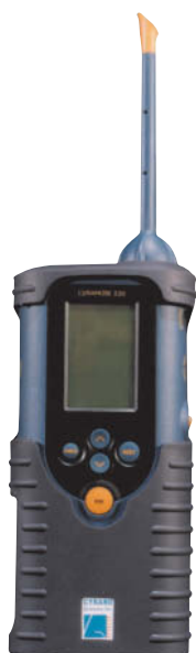
FIGURE 33.9 The Cyranose 320. The electronic nose may find uses in the food industry, animal husbandry, law enforcement, and medicine. [Courtesy of Smiths Medical.]
