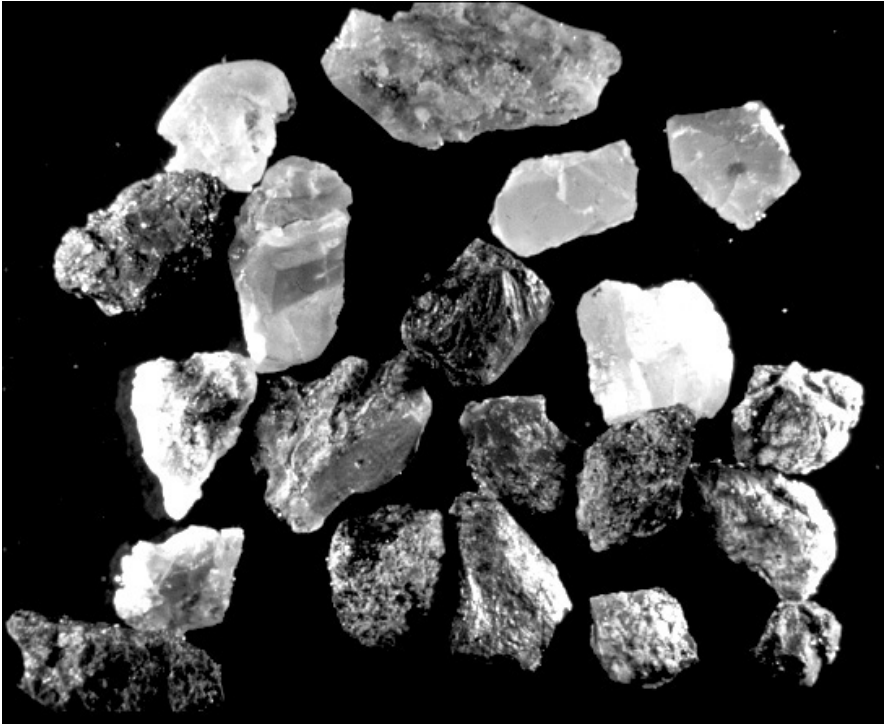
Figure 13-2. Impact diamonds (transformed from graphite flakes) from the Popigai crater, Siberia. The largest grains in this image measure up to 4 mm in size.
