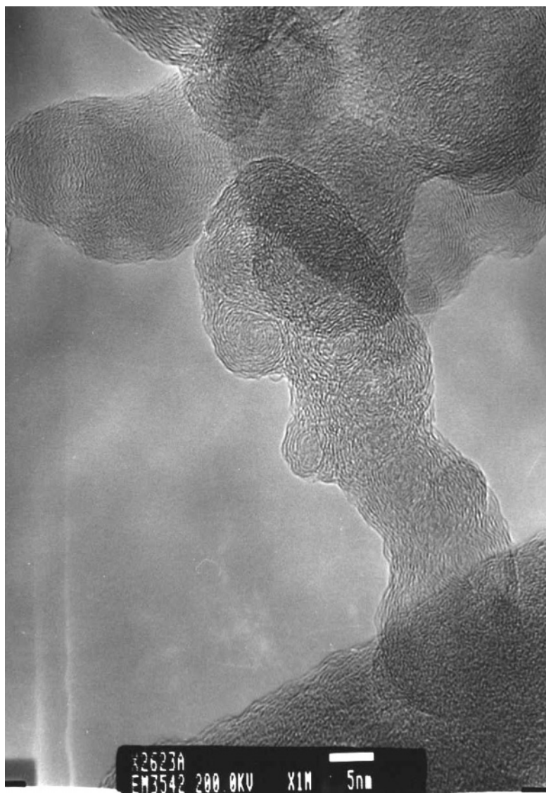
Figure 5.4. HRTEM of furnace carbon black. Note the turbostratic arrangement of the graphene sheets together with the presence of onion-like carbon nanostructures and other curved surfaces.
