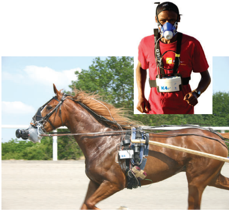
FIGURE 9.3 Modern telemetry devices permit information on O_2 consumption to be radioed from a freely moving subject. In the cases shown, the rate of O_2 consumption is measured using the principle of open-flow respirometry (see Box 7.4). Valves in the mask allow the subject's breathing to cause a measured stream of air to flow through the mask. An O_2 probe measures how much O_2 is removed from each unit of volume of the flowing air. The device has been used to study racehorse performance and the energetics of running in Kenyan athletes (inset). (Courtesy of Marco Brugnoti and Cosmed S.r.l.)
