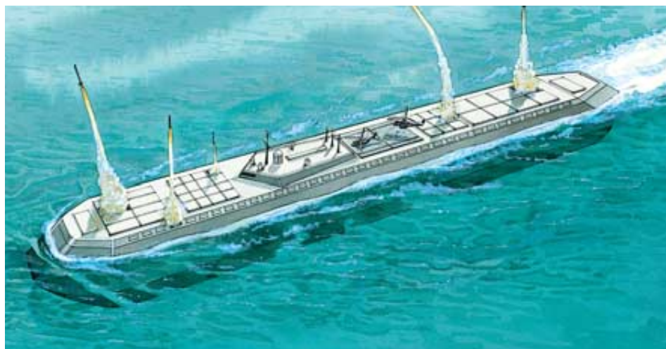
ARSENAL SHIP, with a design perhaps based on that of commercial tankers, could carry hundreds of missiles. The semisubmersible vessel might one day play a strategic role—deploying weapons to their targets—that now is filled by the airplanes on a carrier.
