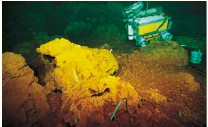
PISCES V SUBMERSIBLE (above, left) is lowered from its support vessel, the Ka'imikai-o-Kanaloa . Ocean-bottom observatory (above) has a time-lapse video camera on top, a seismometer to the right and temperature probes, which are inserted into hot-water vents.
