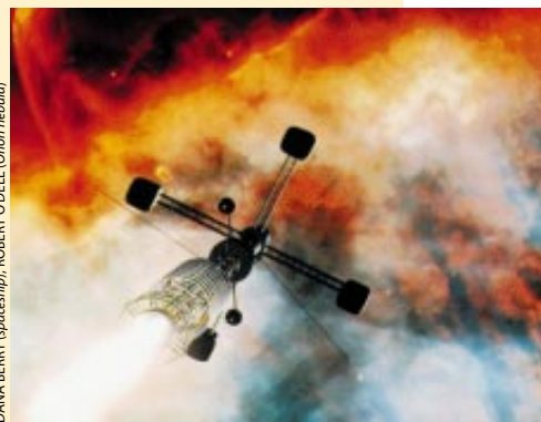
HUMAN-PILOTED interstellar spaceship would have a rotating structure in front, to simulate gravity in four compartments.
