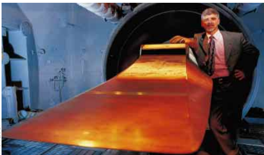
TO THE TEST: Charles McClinton, a NASA engineer, will soon learn whether scramjets can indeed fly. An unmanned prototype (a full-scale replica is shown here, upside down) is scheduled for a flight test at Mach 7 in spring 2000.
