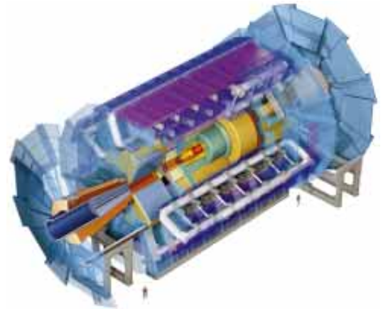
COLOSSAL CAVITY: The 6,600-ton ATLAS detector ( below ), now being assembled for the Large Hadron Collider, will be housed in a chamber large enough to fit a six-story building ( top left ); the entire assembly will be more than 300 feet below ground level. The ATLAS detector is one of four being built for the LHC; work is also in progress on the CMS, ALICE and LHCb detectors ( bottom left ).
