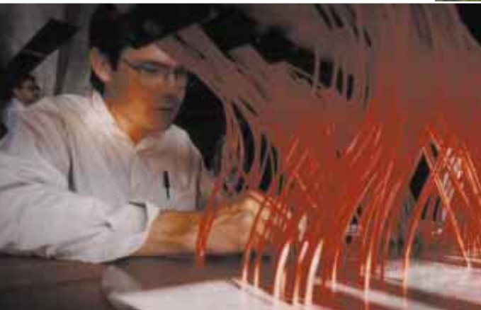
Fiber optics feeding the Sloan spectrograph
