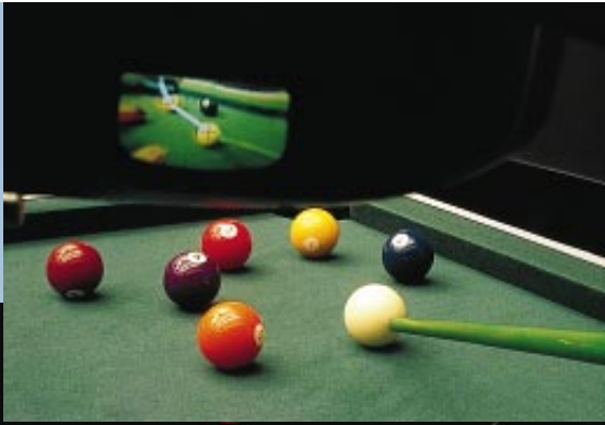
POOL-PLAYING WEARABLE includes a head-mounted camera that records the position of the balls on the pool table. Specially designed software analyzes the possible shots and identifies the easiest one. A heads-up display (inset) helps graduate student Tony Jebara line up the shot.
