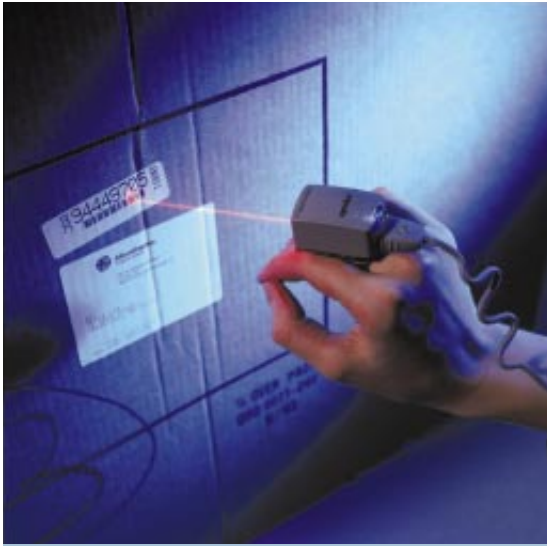
RING WITH BAR-CODE READER is already being sold for use in warehouses and loading docks. The device allows workers to identify the contents of a carton and to read shipping and handling instructions.
