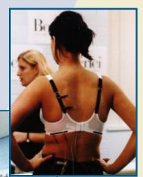
ADJUSTABLE LIFT: Australian researchers test a preliminary mock-up of the Smart Bra, which tightens or relaxes in response to breast movement.
