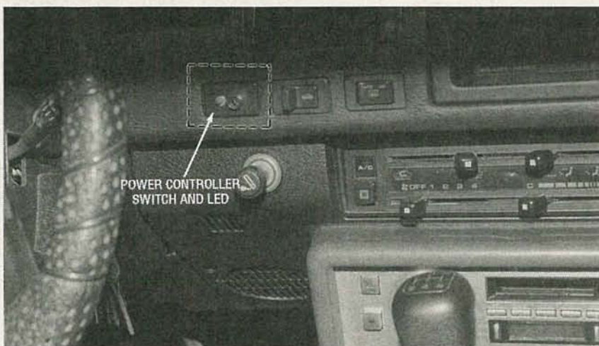
FIG. 2—THE AUTHOR DESIGNED the power controller for a pair of quartz halogen lights that he added to his car. The lights are controlled from a tiny pushbutton switch blended into the dashboard.
