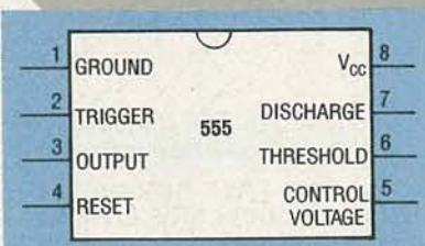
FIG. 1—PINOUT DIAGRAM OF THE 555.
