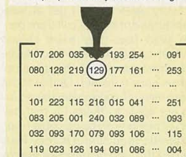
FIG. 2—A DIGITAL IMAGE is nothing but an array of numbers. Digital image processing takes those numbers and replaces them with other numbers following a rule or set of rules. While there is a stunning variety of uses for digital image processing tricks and techniques, two of the most important involve gamma correction and histogram equalization.
