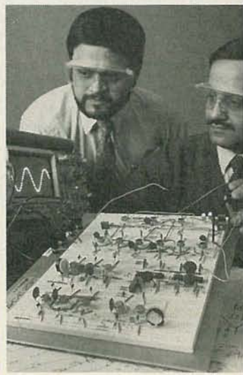
ENGINEERS MANUEL D'ABREU and ABHIJIT CHATTERJEE set up a fault-tolerant circuit breadboard for testing at GE's Research and Development Center.
