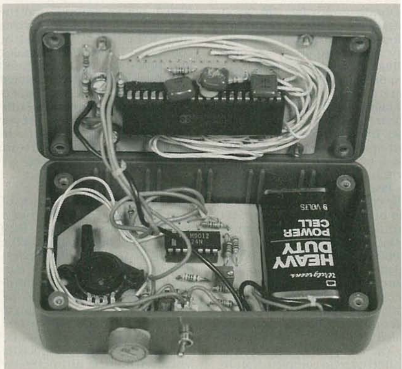
FIG. 6—HERE'S THE AUTHOR'S PROTOTYPE. Notice the four wires that connect the analog and digital boards together.
