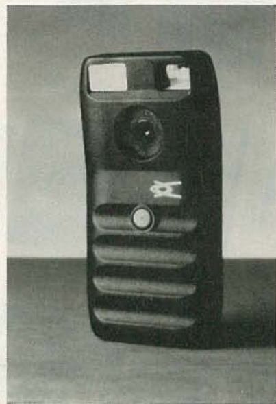
FIG. 1—DYCAM'S MODEL 1 digital camera stores 32 shots, each with a resolution of 376 x 240 x 256 gray levels. It's a harbinger of the future for PC-based digital imaging.
