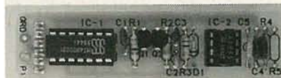
FIG. 15—THE COMPLETED EPROM board. A six-pin female connector (J1) on the solder side mates with P4 on the main board.
