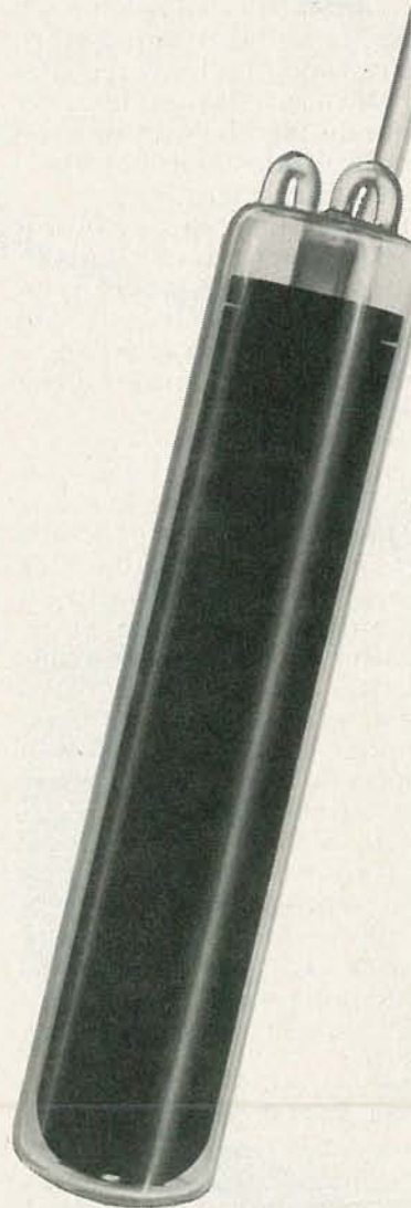
FIG. 2—FIXED POINT CELL. The graphite crucible, visible through the quartz enclosure, contains a high-purity metal. (Courtesy of YSI Inc.)
