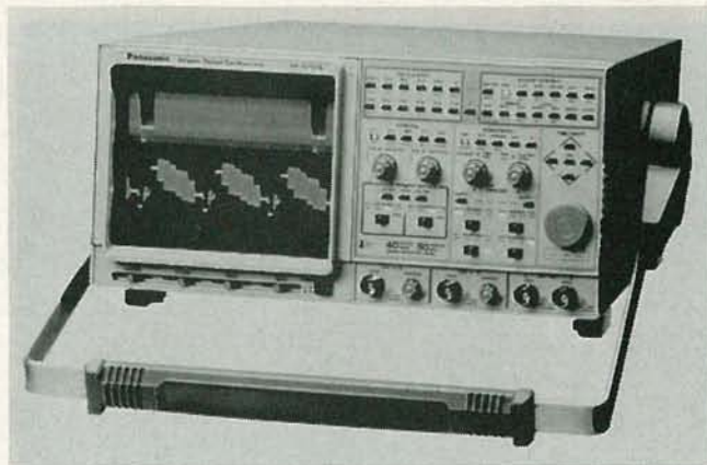
PANASONIC MODEL VP-5720A is a 2-channel, 50-MHz repetitive bandwidth DSO featuring a 15-MHz single-shot bandwidth and a 40 Ms/s sampling rate. It has a 8K x 3 memory storage and an expandable memory option.
