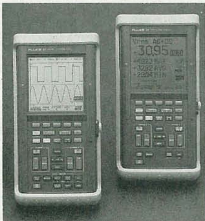
FLUKE'S HANDHELD SCOPEMETER models 95 and 97 feature 50-MHz dual channel, 25 Ms/s sampling rate with auto-set. A combination DSO and DMM, these instruments are ideal for rugged field use. Model 97 also has a sine wave or square wave signal generator output with optically isolated RS-232C remote control operation.
