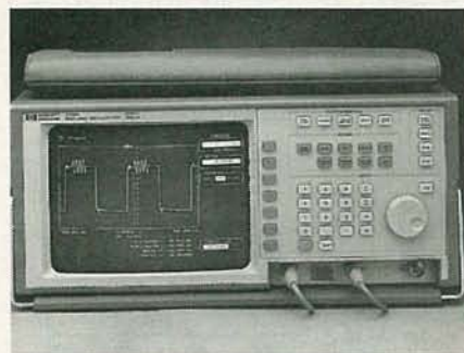
HEWLETT PACKARD'S SPECIAL —a dual channel, large screen digital (only) 54510A scope that digitizes 2 channels at 1 gigasample per second (Gs/s) with 8-bit vertical resolution.
