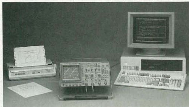
TEKTRONIX' ANALOG 2252 4-channel scope with a 12-bit A/D converter, an Epson FX-series printer, and an IBM remote PC all combined to form a complete recording package.
