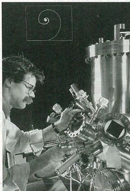
BELLCORE RESEARCHER BILL QUINN grows aluminum gallium arsenide crystals for use in semiconductor materials and devices, using an experimental process that corrects small errors in material composition as they occur, resulting in the world's most precise crystals.
