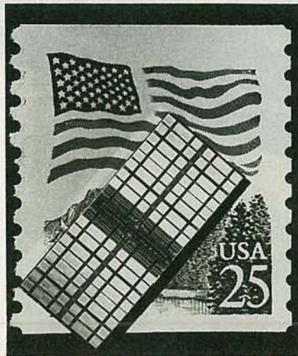
IBM'S 16-MEGABIT MEMORY IC, shown on a postage stamp, can read all of its 16,777,216 bits of information in \frac{1}{25} of a second, which is several times faster than the blink of an eye.
