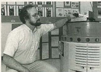
DR. RONALD ARKIN ADJUSTS the vision system that "George," Georgia Tech's specially modified materials-handling robot, uses to navigate to its objective.
