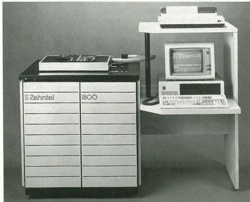
FIG. 4—ZEHNTel 1800 BOARD TESTER. A PC serves as controller, and the UUT fixture is on the console at left. Note the vacuum hose to the right. The 1800 is prewired for 640 analog/digital test points.
