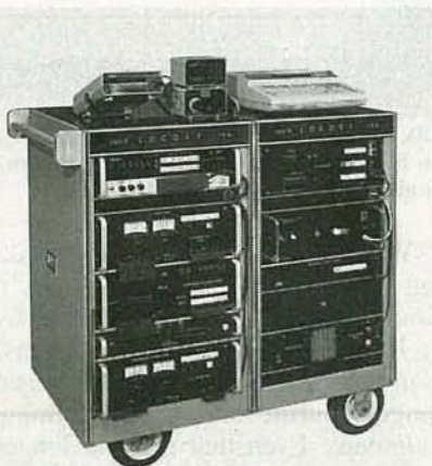
FIG.6—THE JULIE RESEARCH LABORATORIES LOCOST 106. This version automatically calibrates test equipment and calibration standards. The desktop-computer controller is at top right.
