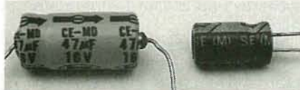
FIG. 3—THE LEADS of an axial-lead capacitor (left) extend along its axis; those of a radial-lead one (right) align with a radius.
