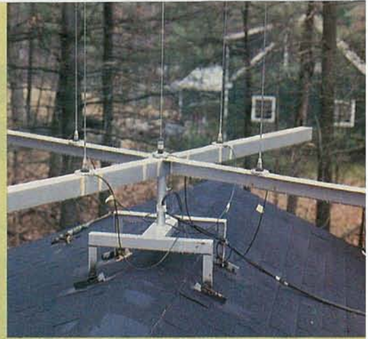
FIG. 6—DIRECTION FINDING using Doppler System's four matched quarter-wave whips, shown in (a), are supported on magnetically mounted bases for mobile operation. In (b), four collapsible antennas are mounted on a sturdy platform, on top of the author's roof.
