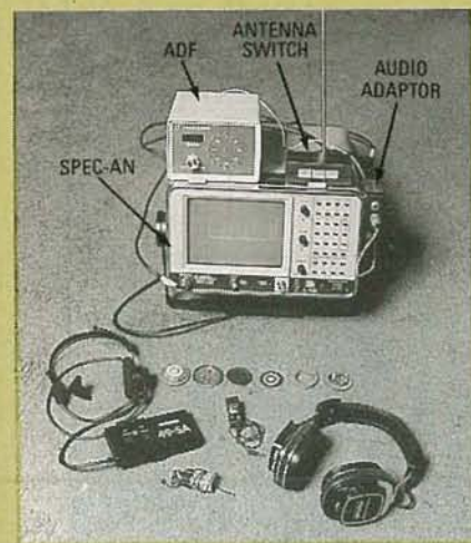
FIG. 5—HERE'S YOUR PERFECT sleuthing setup: a spectrum analyzer, automatic direction-finder, antenna switching box, and headphone audio-adaptor to listen privately to clandestine transmissions.
