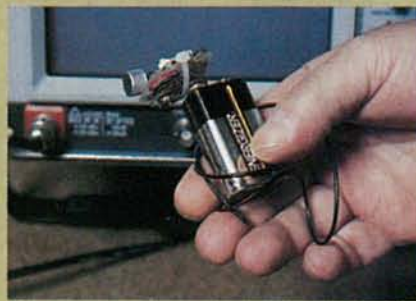
FIG. 1—THESE ARE CLANDESTINE radio bugs. In (a), a parasitic phone-tap is shown disassembled. In (b), a Radio Shack FM-transmitter (part No. 33-1076) can be conveniently dropped behind the cushion of a chair. In (c), this tiny FM transmitter can be hidden in a kitchen cabinet.
