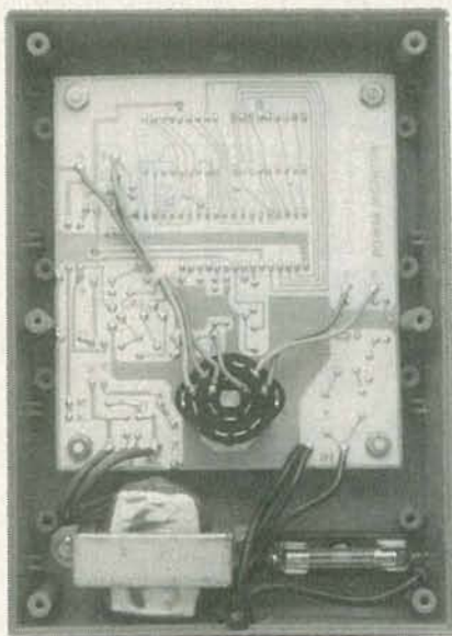
FIG. 4—VOLTS-NOISE SWITCH S1 is mounted on the foil side of the PC-board. Its connections are tack-soldered to the appropriate solder pads.
