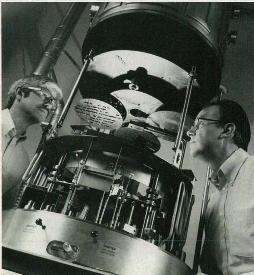
ELECTRON-BEAM EVAPORATION SYSTEM is being prepared to deposit a zirconia buffer and superconducting film on silicon chips by co-developers Larry G. Turner and Dr. Antonio Mogro-Campero.
