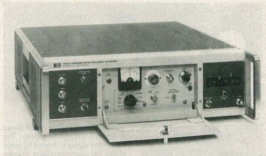
FIG. 5—A RUBIDIUM-VAPOR FREQUENCY STANDARD. This device is manufactured by Hewlett Packard.
