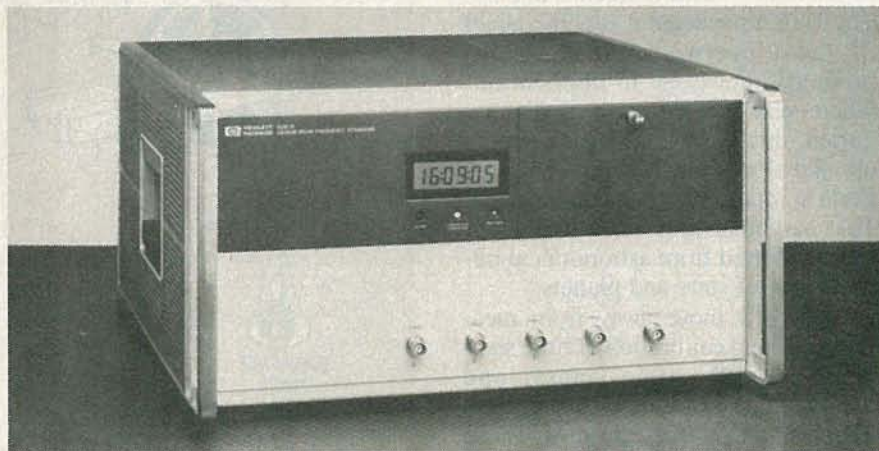
FIG. 3—A CESIUM-BEAM FREQUENCY STANDARD. This device is manufactured by Hewlett Packard.
