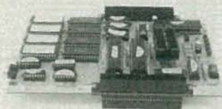
THE FINISHED PROM/RAM DISK. Note the ZIF socket near the center of the unit.
