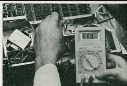
The power supply is assembled in the main unit of the computer. You check out keyboard connections and circuits with the digital multimeter included for training and field use.
