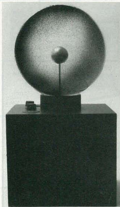
FIG. 7—THE COMPLETED DISPLAY should resemble this author's prototype. Be sure that the globe base you select can support the size of plasma globe that you intend to use.
