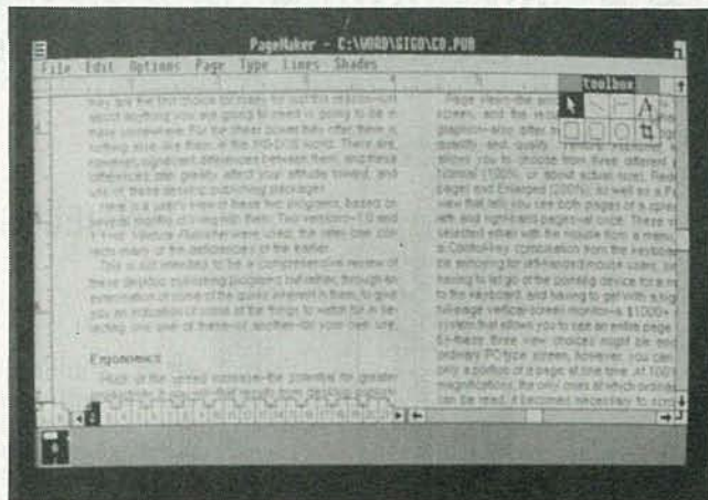
FIG. 5—PAGEMAKER PROVIDES A GRAPHICS TOOLBOX (shown in the upper right corner) that allows you to create lines, circles, and boxes, and to crop and scale graphics images.
