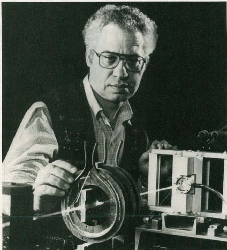
GIAN P. FLETCHER, ARGONNE NATIONAL LABORATORY scientist, with the polarized-neutron reflectometer that could lead to improvements in magnetic recording.
