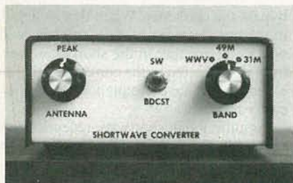
FIG. 7—THE COMPLETED CONVERTER. If you wish, follow the design shown here when laying out your front panel.
