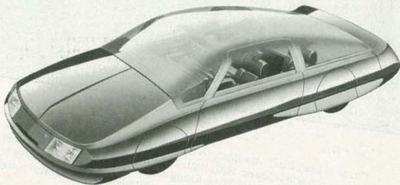
THE ALL-GLASS TOP OF FORD'S 2001 MODEL is flush with the body, giving the car excellent aerodynamic performance.
