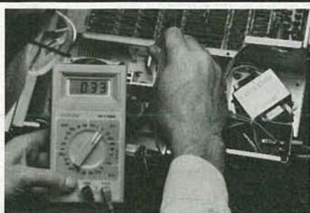
The power supply is assembled in the main unit of the computer. You check out keyboard connections and circuits with the digital multimeter included for training and field use.
