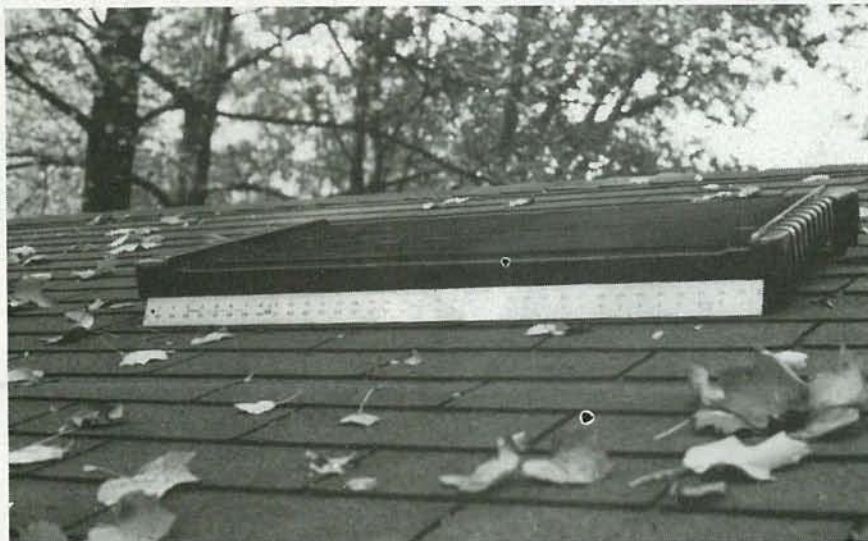
FIG. 1—THIS PROTOTYPE LIMPET GENERATOR, installed on a rooftop in Maryland, is but six inches high.
