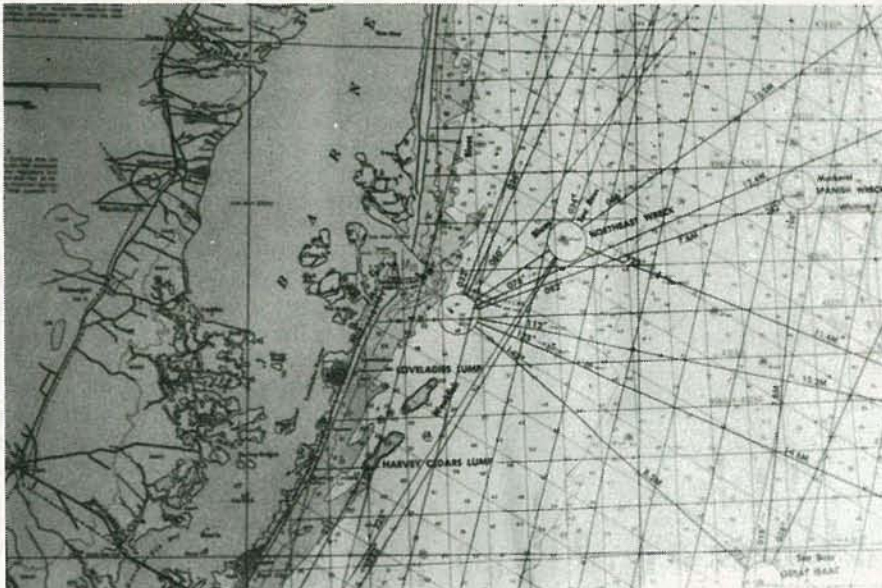
FIG. 3—A NAVIGATION CHART shows the Loran-C time-difference lines for the chains that can be received within a localized area.
