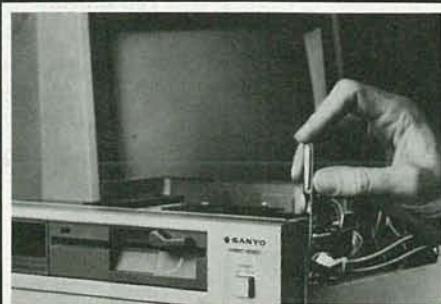
Next, you install the disk drive. You learn disk drive operation and adjustment, make a copy of MS-DOS operating disk and begin your exploration of the 8088 CPU.
