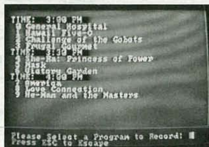
THE VIDEO RESOURCE MANAGER (VRM) was installed in the author's home for three months for testing. It allowed us to share video resources among four TV sets via remote control. The remote controllers were based on Touch-Tone -like keypads.
