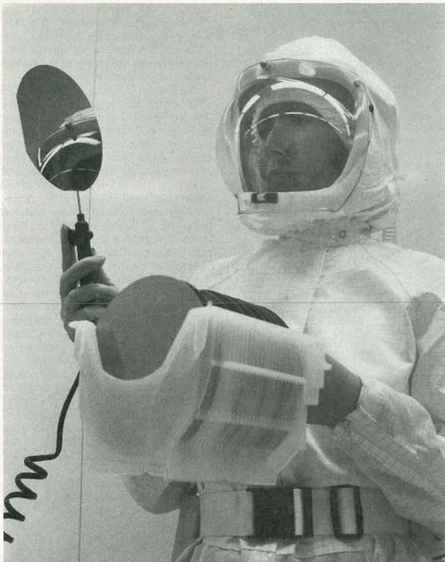
FIG. 3—ULTRA-CLEAN AIR is required in VHSIC manufacturing. A single air-borne particle could ruin one of the 240 VLSI and VHSIC chips on the 6-inch wafer.
