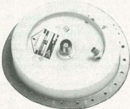
FIG. 10—PERFORMANCE OF AN L-BAND antenna can be measured with a TDR.
