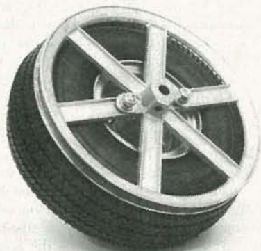
FIG. 7—IF BOLTED TOGETHER PROPERLY, the wheel and pulley assembly will resemble the one shown here.
