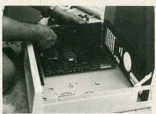
FIG. 3—TO ALIGN THE MOTHERBOARD, temporarily install a couple of expansion cards.
