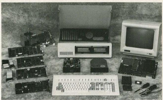
FIG. 1—EVERYTHING YOU NEED to assemble a complete computer system. Turn to page 108 for a description of each component.
