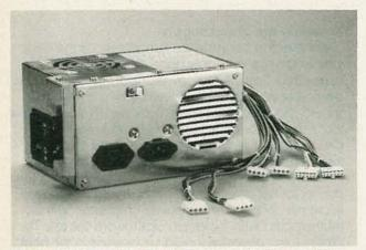
FIG. 5—THE POWER SUPPLY. Note the side-mounted power switch and the numerous power connectors.
