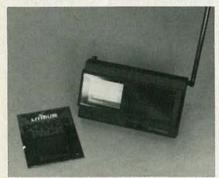
FIG. 12—SINCLAIR POCKET TV uses a P500 for power.
