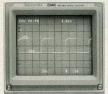
FIG. 2—PEAK-TO-PEAK MEASUREMENT shows the entire 1 to 0 voltage swing of a digital waveform.
