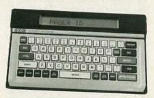
FIG. 16—THE *TC200* is a portable telecomputer that provides 8K of RAM and a built-in modem. It's powered by a *P500*.
