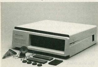
FIG. 6—THE COMPUTER'S CASE has a flip-top lid, which makes system expansion a snap!
